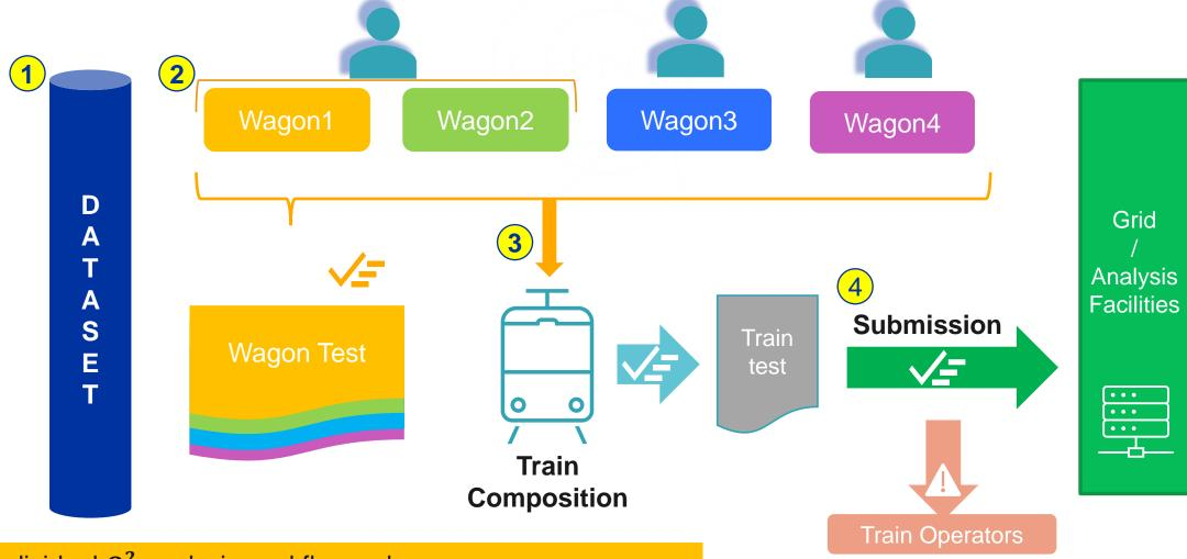
Individual  $O^2$  analysis workflows - known as wagons - are combined into trains to run over the data together
