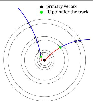
— IU track — track propagated to PV The <u>track parametrization</u> at <u>different radii changes</u>
